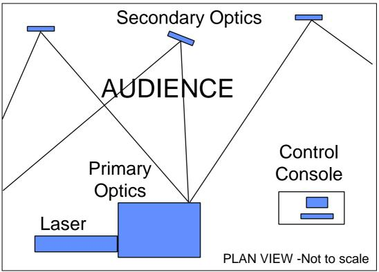
Figure 3.1 Simple Laser Display System
